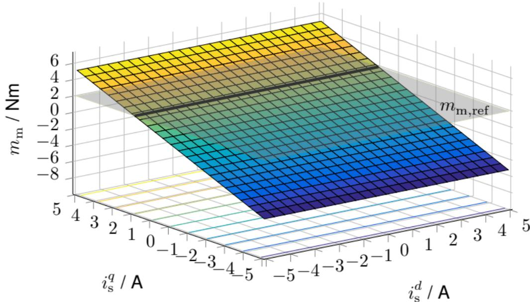
$$m_{m,\text{ref}} \stackrel{!}{=} m_m(i_s^d, i_s^q) = \frac{2n_p}{3\kappa^2} \psi_{\text{pm}} i_s^q \implies \mathbf{i}_{s,\text{ref}}^{dq} := (i_{s,\text{ref}}^d, i_{s,\text{ref}}^q)^\top = \left( 0, \frac{3\kappa^2 m_{m,\text{ref}}}{2n_p \psi_{\text{pm}}} \right)^\top$$
