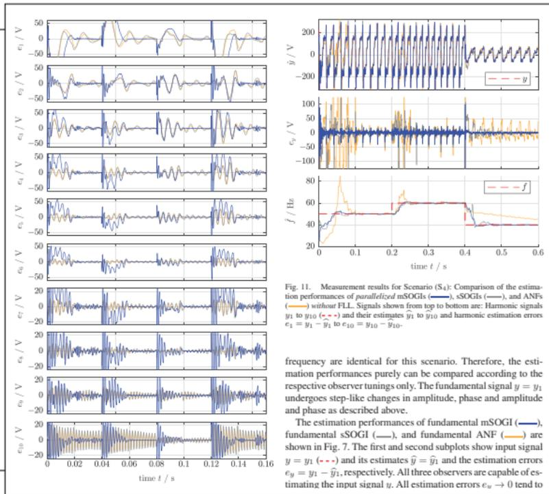
Fig. 11. Measurement results for Scenario (S<sub>4</sub>): Comparison of the estimation performances of parallelized mSOGIs (—), sSOGIs (---), and ANFs (····) without FLL. Signals shown from top to bottom are: Harmonic signals  $y_1$  to  $y_{10}$  (---) and their estimates  $\hat{y}_1$  to  $\hat{y}_{10}$  and harmonic estimation errors  $e_1 = \hat{y}_1 - y_1$  to  $e_{10} = \hat{y}_{10} - y_{10}$ .
