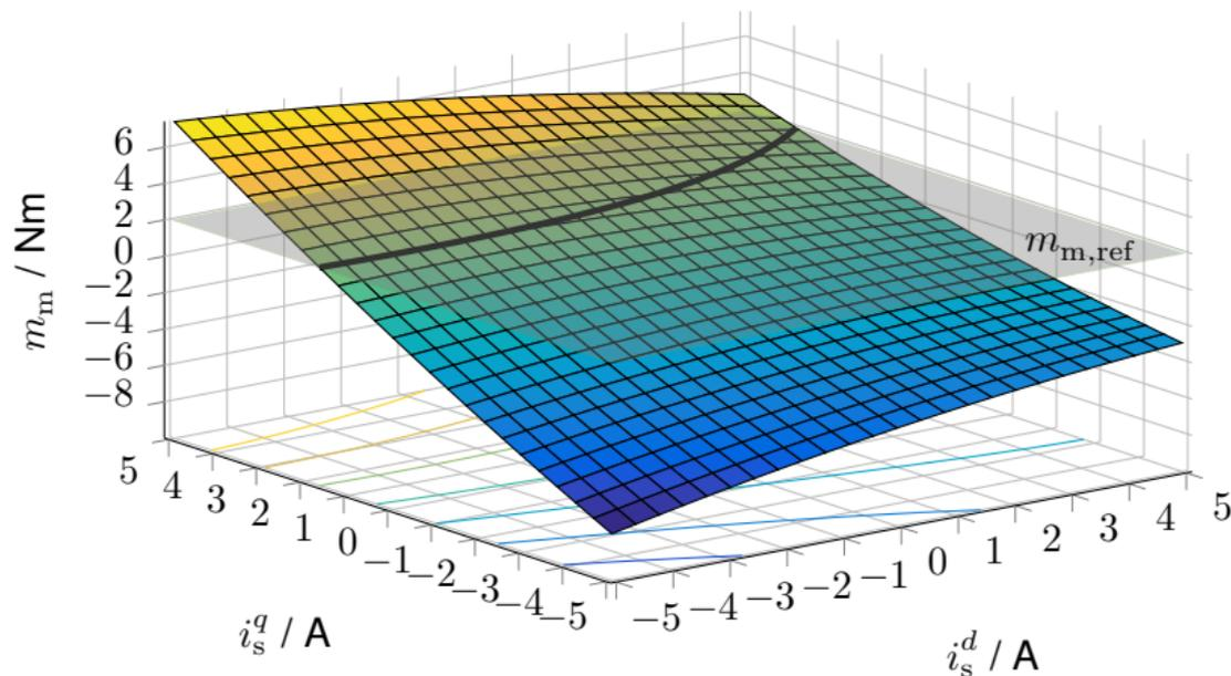
$$m_{m,\text{ref}} \stackrel{!}{=} m_m(\mathbf{i}_s^{dq}) = \frac{2n_p}{3\kappa^2} \left[ \tilde{\psi}_{\text{pm}} i_s^q + (\tilde{L}_s^d - \tilde{L}_s^q) i_s^d i_s^q + \tilde{L}_{s,m} ((i_s^q)^2 - (i_s^d)^2) \right] \implies \mathbf{i}_{s,\text{ref}}^{dq} := (\text{?}, \text{?})^\top$$
