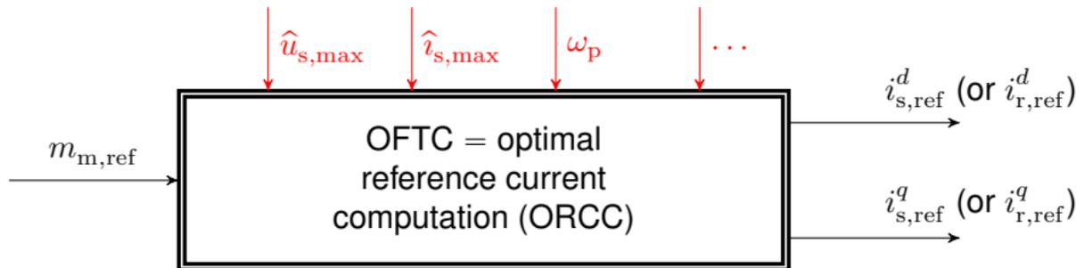
$$\mathbf{i}_{s,ref}^{dq}(m_{m,ref}, \hat{u}_{s,max}, \hat{i}_{s,max}, \omega_p, \dots) = \begin{pmatrix} i_{s,ref}^d(m_{m,ref}, \hat{u}_{s,max}, \hat{i}_{s,max}, \omega_p, \dots) \\ i_{s,ref}^q(m_{m,ref}, \hat{u}_{s,max}, \hat{i}_{s,max}, \omega_p, \dots) \end{pmatrix}$$
