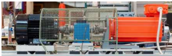
Reluctance SM (RSM) and Permanent-magnet SM
