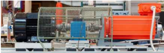
Reluctance SM (RSM) and Permanent-magnet SM
